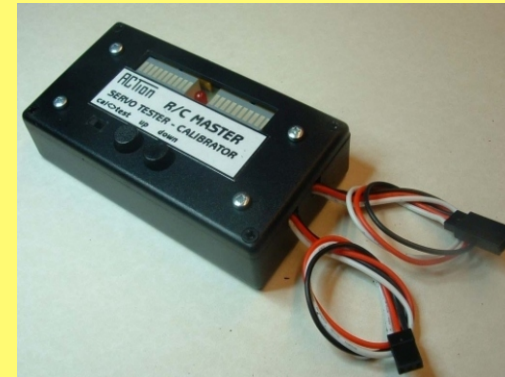
PICTURE 9: Fit into case and add label
