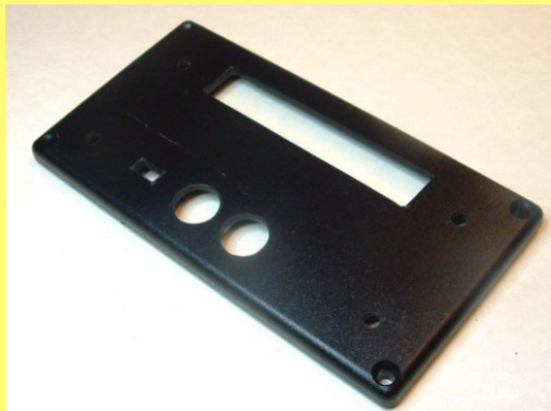
PICTURE 7: Snip out waste and file cut-outs back to lines. Deburr holes
